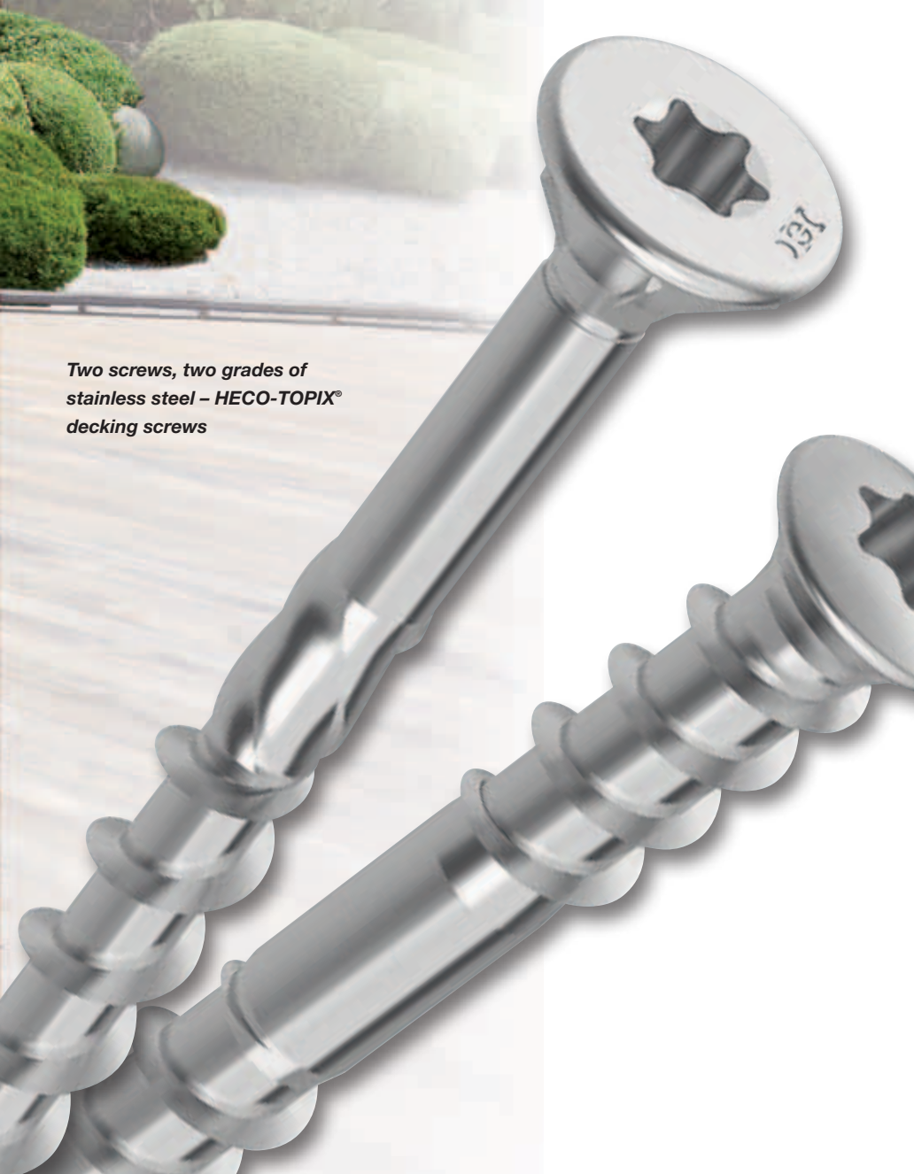
A4 stainless steel should be used when particularly high demands are placed on the ability to resist corrosion; such as for poolside and seaside decking as well as when highly tannic woods are used.
