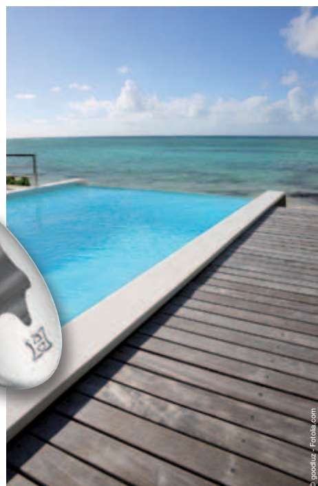
A4 stainless steel should be used when particularly high demands are placed on the ability to resist corrosion; such as for poolside and seaside decking as well as when highly tannic woods are used.
